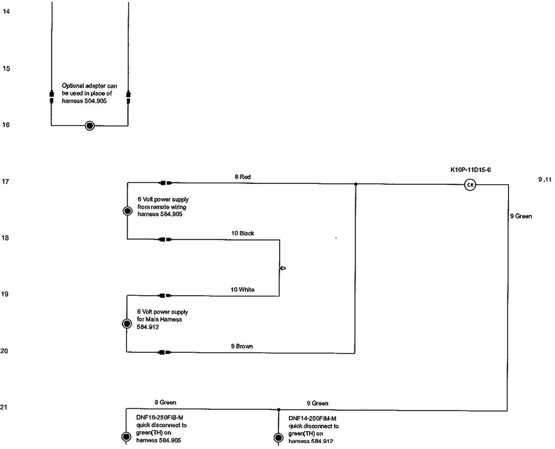
**If any of the original wire as supplied with the appliance must be replaced, it must be replaced with type 18 AWG, 105 C, Deca Cables p/n 74-623 or its equivalent.**
