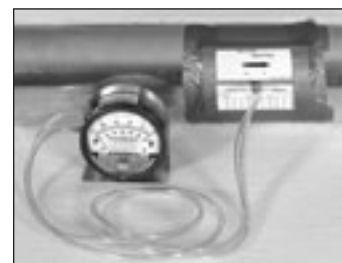
Seal Air flow grid in duct with duct tape.
